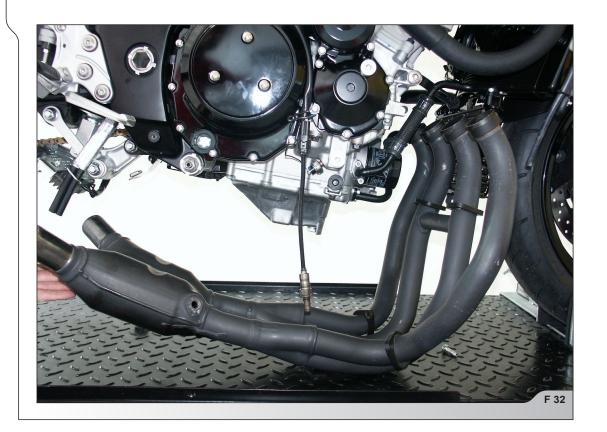
12. Unscrew and remove the chassis hanging bracket of stock headers (F 33, 34). For Racing twin exhaust only: replace the stock chassis hanging bracket of stock headers with special Akrapovic bracket (tightening torque 22Nm/16ftlb).
