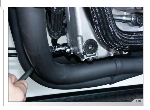
9. Unscrew and remove the lambda sensor (F 28, 29).
