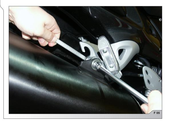
5. Remove the mufflers and the gaskets (F 06, 07, 08).
