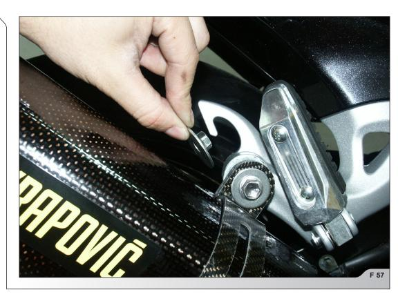
10. Tighten the bolt(s) on the carbon-fiber clamp(s)/stock muffler bracket joint(s) (F 58). Make sure the link pipe or muffler is not touching the frame or any other part of the motorcycle.
